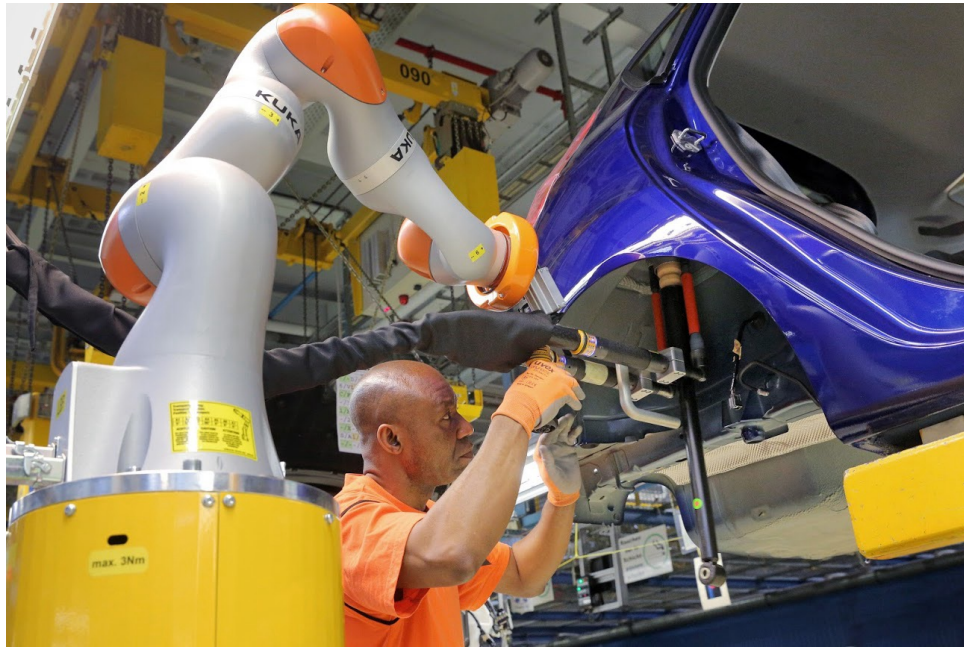
FIGURE 1: A cobot application at a Ford Motor Company’s assembly plant in Cologne, Germany. In the application, the cobot carries a heavy, air-powered tool, which the worker positions during the installation of shock absorbers in Ford Fiesta model cars. (Copyright: Ford Media Center , permission pending.)
